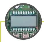
The integrated display facilitates device programming. A password can be set to further guarantee maximum security where there is a risk of tampering by unauthorised persons; this gives the receiver a functional level on a par with the most sophisticated Benincà control units.
