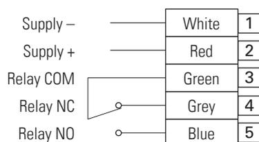
Stripping length min. 8.5 mm (solid or flexible wire)
