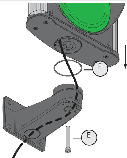
When the bottom cover is closed, fasten the body to the lower bracket previously fixed (Page 9), by means of the special self-tapping screw [E], paying attention to the repositioning of the OR ring [F]
