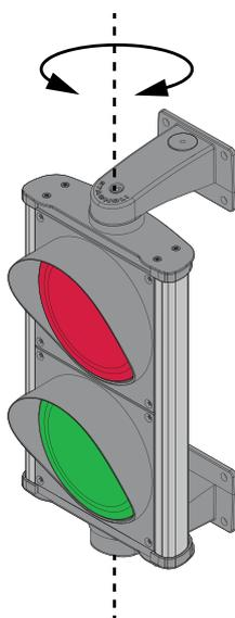
Once completely installed, the body can be rotated simply by loosening the brackets' fixing screws.
