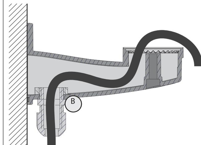
Once the correct routing of the cable has been set, fix the bracket to the wall using the suitable screws and screw anchors.
