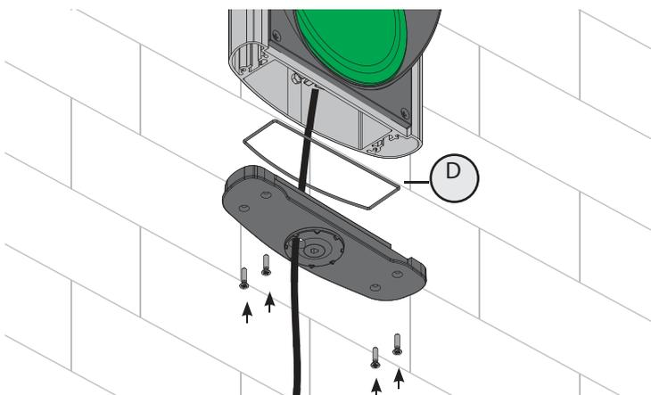
When the wiring is finished, close the cover ensuring that the OR ring is repositioned [D]
