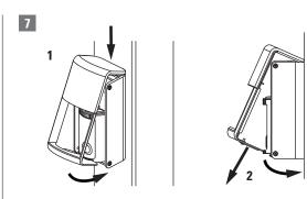
First hook the front cover on the top of the base and then snap it onto the base while pulling down.
