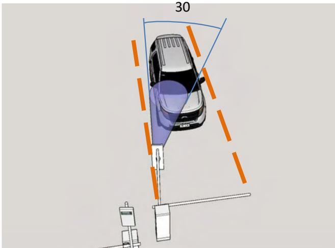
The antenna is transmitting via cone of approximately 30 degrees.
