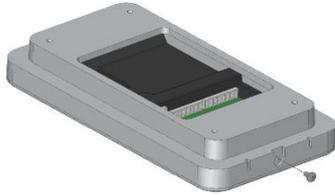
**Step 2-** Separate the panel from the back cover.
