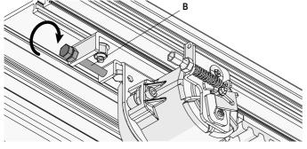
Tighten the belt using screw B.
