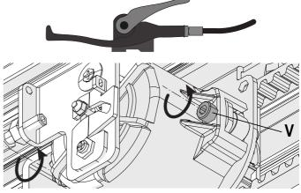
Repeat the operation if the doors open more than planned (+/- 2mm ~) N.B. Leave a couple of mm in range between the two doors.
