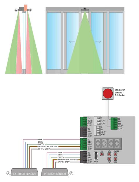
Connect the sensor, using the cable supplied, to the terminals of the electronic control as follows:
