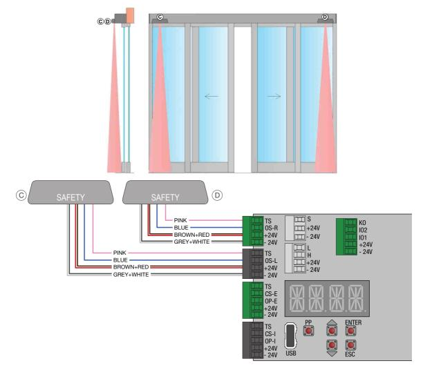
Connect the sensor, using the cable supplied, to the terminals of the electronic control as follows:
