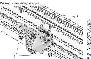
Fasten the electric lock/belt return kit using screws A.
