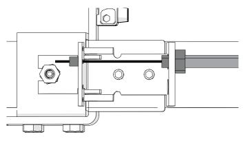
Fasten the manual unlocking lever in the desired position using the hole F.
