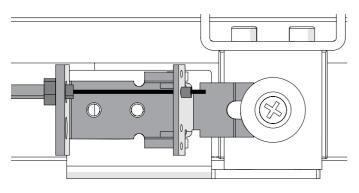
Fasten the manual unlocking lever in the desired position using the hole F.
