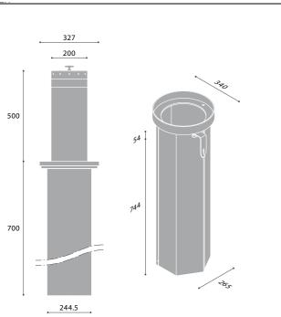
The embedded un-lock device is equipped with waterproof stainless steel plug
