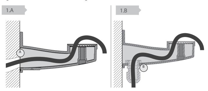
Once the correct routing of the cable has been set, fix the bracket to the wall using the suitable screws and screw anchors.
