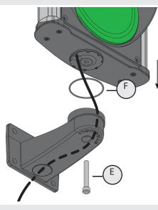
When the bottom cover is closed, fasten the body to the lower bracked previously fixed (Page 9), by means of the special self-tapping screw [E], paying attention to the repositioning of the OR ring [F]
