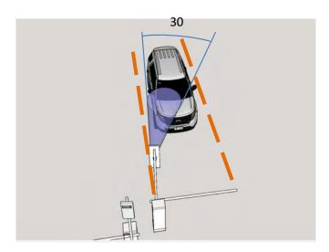
The antenna is transmitting via cone of approximately 30 degrees.
