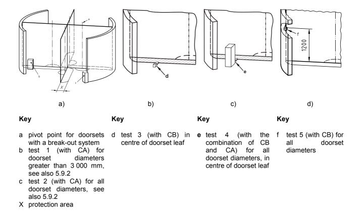
Figure C.9 — Revolving doorset, four leaves
