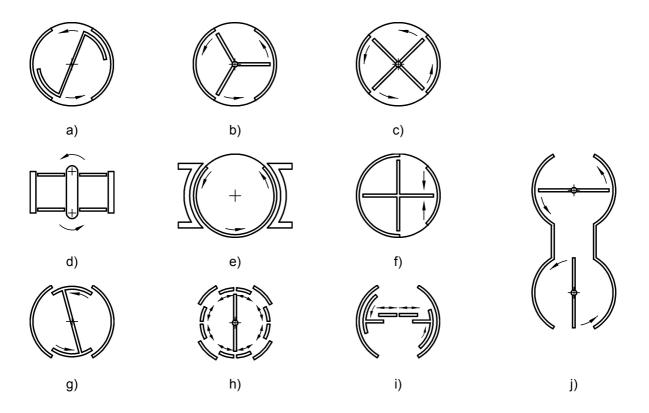
Figure 1 — Revolving doorsets
