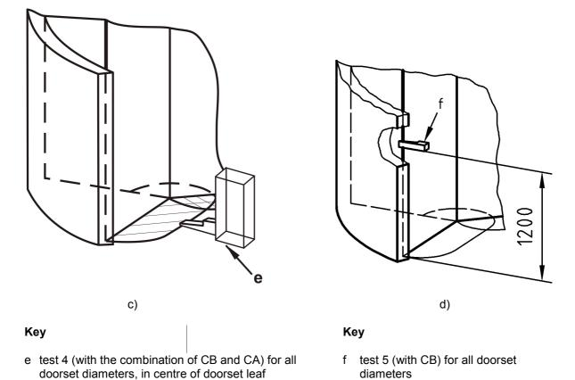
Figure C.7 — Revolving doorset, two leaves
