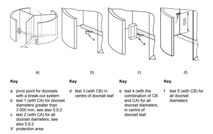
Figure C.8 — Revolving doorset, three leaves
