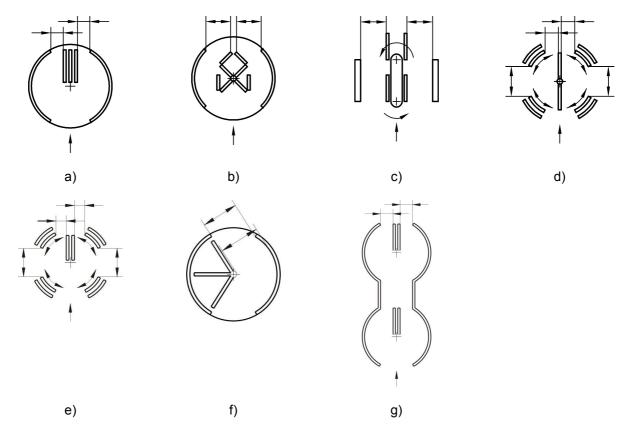
Figure 6 — Typical emergency escape position of power operated revolving pedestrian doorsets
